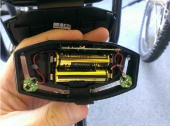
To change the batteries on the front light, press down gently on the tab at the bottom to release the lens. Then lift it clear of the housing. Behind the lens there are 2x AA batteries. To operate the light, press the button located on the top of the light, to turn it on, press it again to flash, and once more to turn it off.
