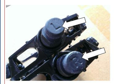
Please note that the thread for the left pedal is reversed and so it tightens anti-clockwise.
