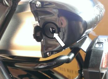
To charge the battery, simply lift the weatherproof cover and connect the charger to the socket and then plug the other end into a regular mains socket. On the charger is a small light which is red while charging. When charging is complete, this light will turn green.
