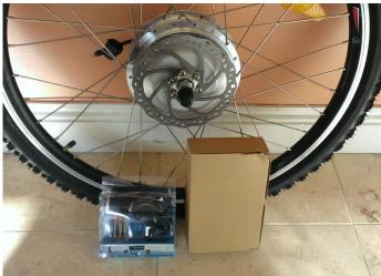
Once you have the bike out of the box, detach the wheel and remove all of the remaining packaging (if applicable). This model sometimes comes 95% assembled meaning that the front motor wheel and torque arms are already fitted, if this is the case you can skip those sections.
