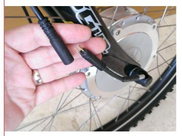
When attaching the motor cable, ensure that the arrow on each side of the connectors line up with each other, otherwise you may damage the connector.
