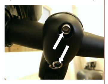
To adjust the **rotation** of the handlebars (to ensure that the angle of the brakes/display etc. is correct), loosen the front-most bolt on the underside of the handlebars as shown above right. Rotate the handlebars into the desired position and then re-tighten the bolt. Check the adjacent bolt is sufficiently tight and tighten if required.
