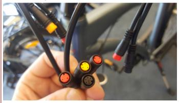
There is an arrow on each of the connectors, ensure that you line up the arrows and then push them firmly together.
